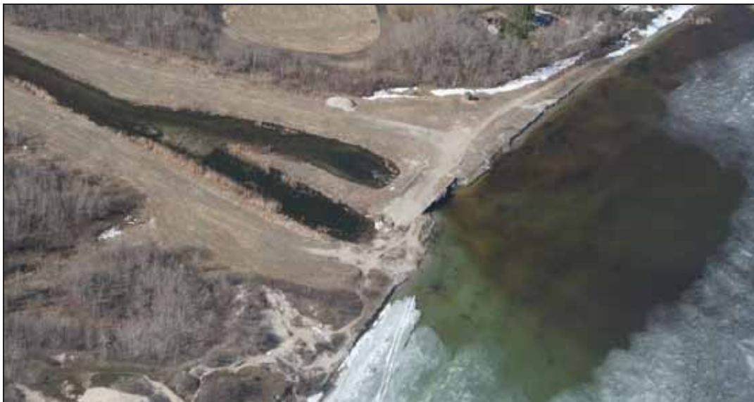
3-culvert outlet structure and overflow spillway in SW corner of Good Spirit Lake
